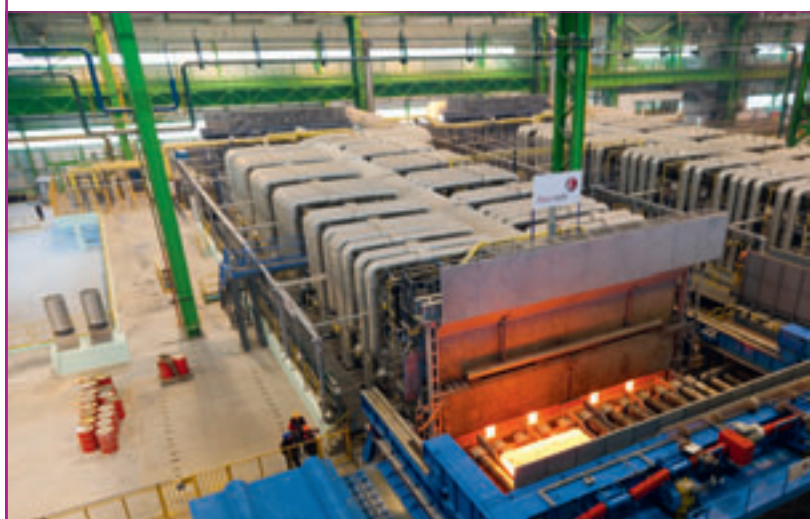
The first hot slab from Fives’ Digit@l Furnace® installed at Mill-5000 of Vyksa Metal Works, OMK
