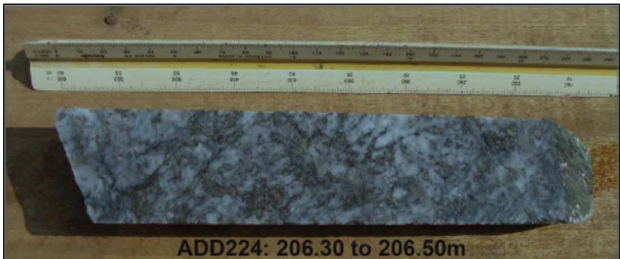
Figure 7-4 Drill Core Sample of Mottled Quartz Vein in Fresh Rock
