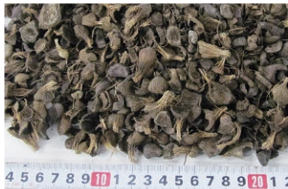
PKS as a fuel for biomass boilers (shell fractions left after oil has been extracted from the oil palm)
