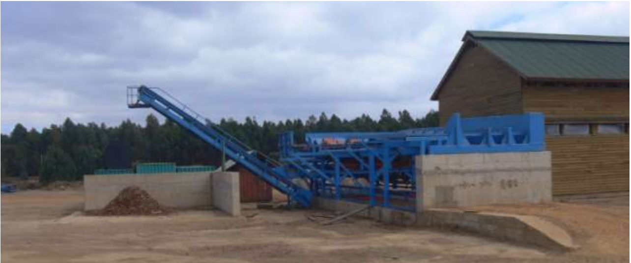
Log infeed with bark outfeed from the debarker to the left. The cleanly separated bark will be used for energy and for soil substrate/ soil compost.
