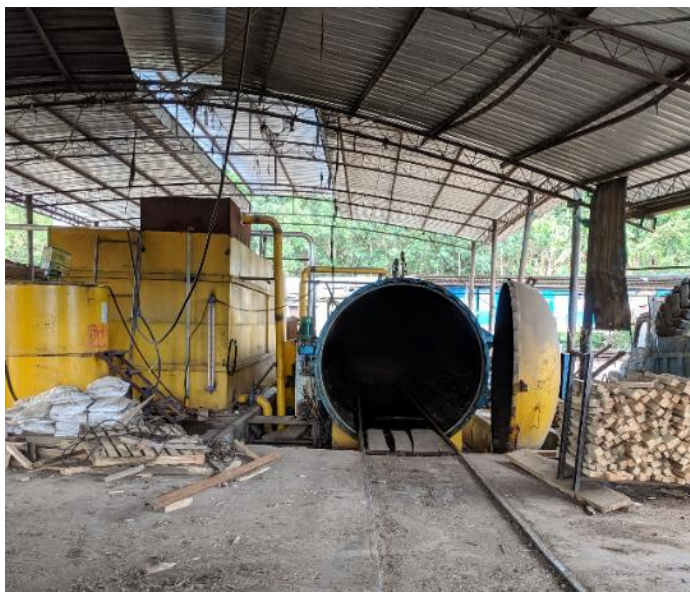
Figure 26: Pressure treating rubberwood for fungal decay
