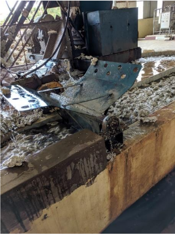
Figure 17: Cup lump washing and shredding
