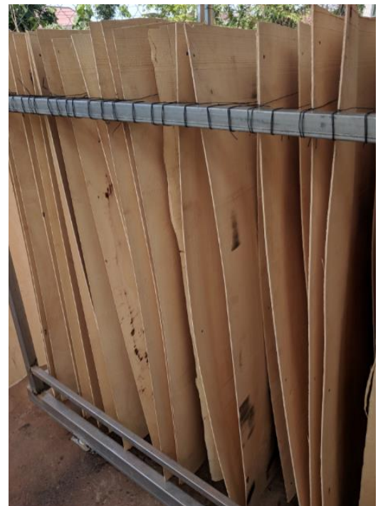
Figure 25: Rubberwood Veneer peeled at NUoL
