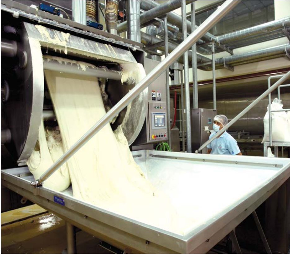
Dough mixer at The Italian Baker's baking plant in Pulau Indah
