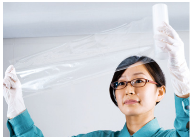
Continuous transparent sheet of cellulose nano-fiber
