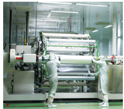
Clean coater at Yamamoto Plant of New Tac Kasei, an optical functional products' manufacturer
