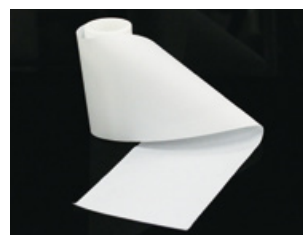
Continuous porous sheet of cellulose nano-fiber
