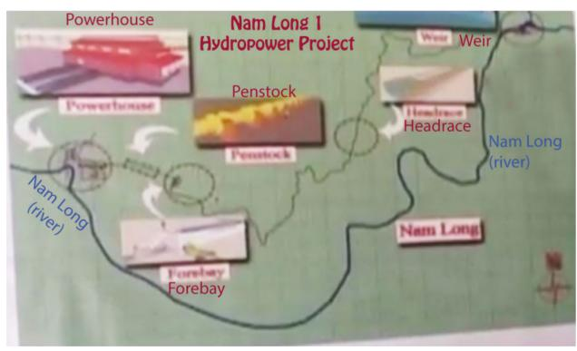
The project is a run-of-river type. The installed capacity of the project is 5 MW. Estimated annual output of 37 GWh (seems a bit high) will be supplied to the local Luang Namtha grid. As of year 2020 this grid is not connected with the main grid of Lao EDL but connected with China Southern Power Grid through transmission lines.
