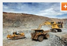
Haul trucks carrying the run of mine ore to the processing facility.
