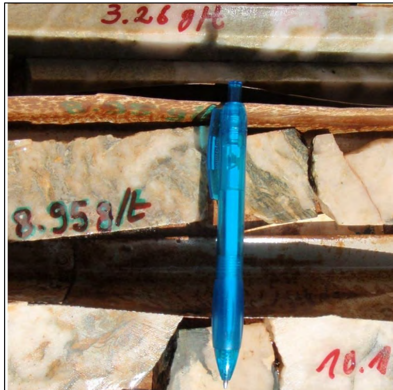
Figure 12.5 Siou Deposit Zone 9 – Mineralized Intercept in Drill Hole WDC 594
