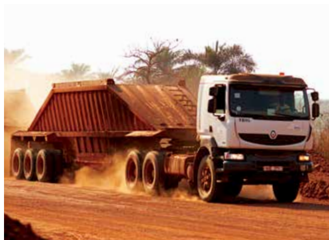
Trucking of concentrate along Marampa's 40km haul road.
