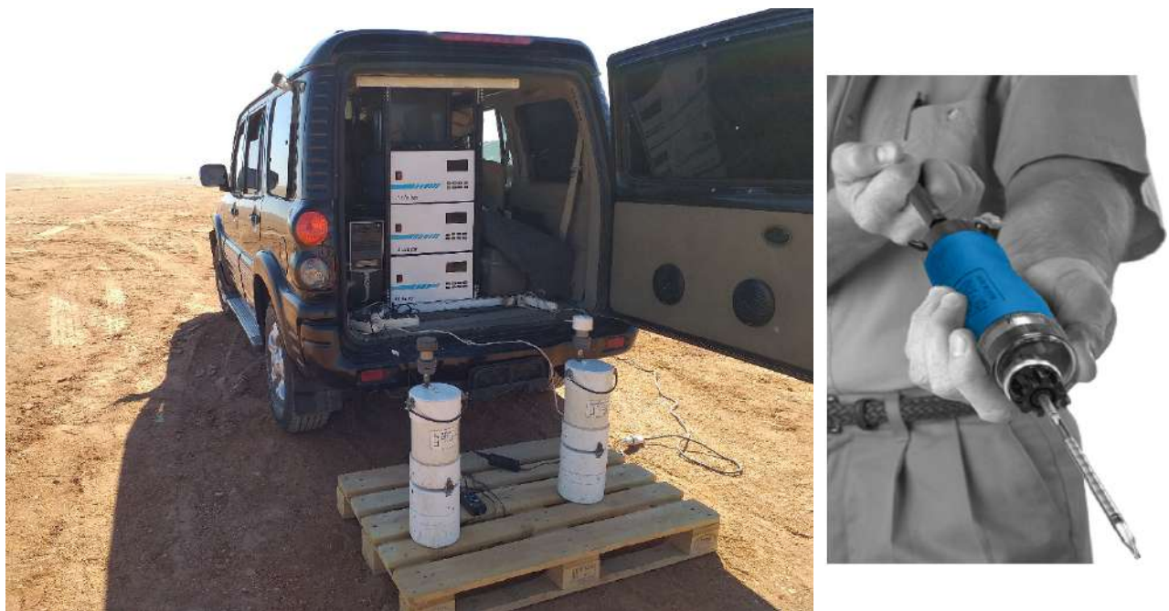
Figure 5-14 Photo of AQ monitoring equipment (left) and ozone colorimetric gas detection tube (right).
