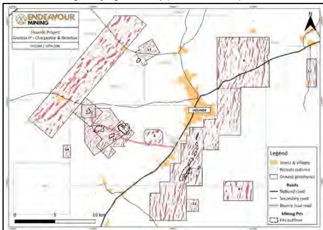
Figure 9-13: Gradient Array IP surveys from 2014 to 2019 - Combined resistivity high / chargeability high worm map (source: Endeavour)
