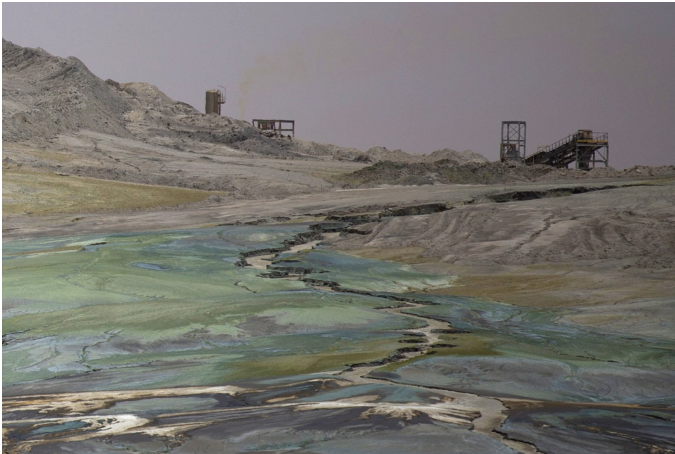
Uranium ore is heap leached with sulphuric acid at Areva's Somair mine in Arlit, September 25, 2013. REUTERS/Joe Penne
