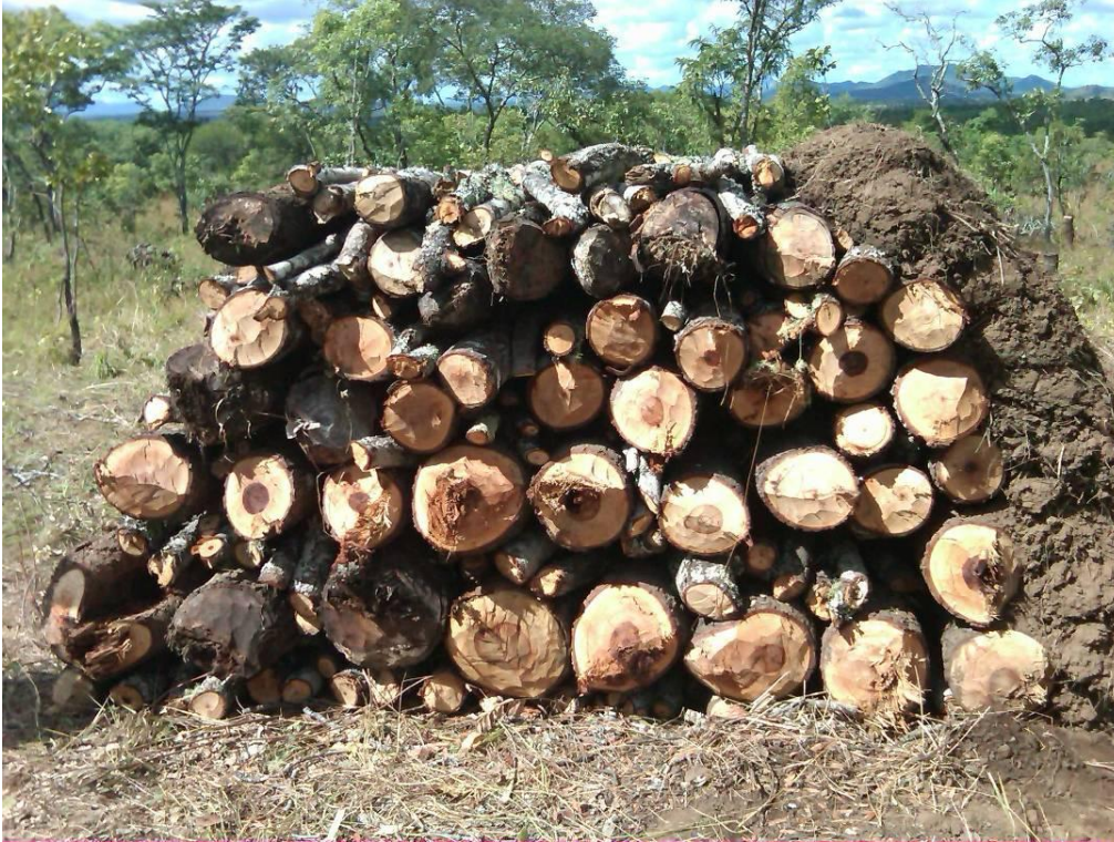
Image 1. Wood stacked and covered with clay. A typical local charcoal kiln. From Malulu unit, NGR
