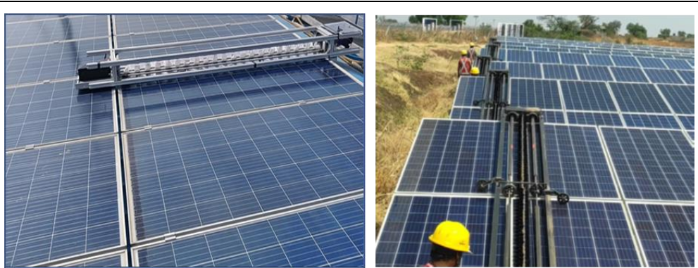
Robotic Dry-Cleaning System at Avaada Sites
