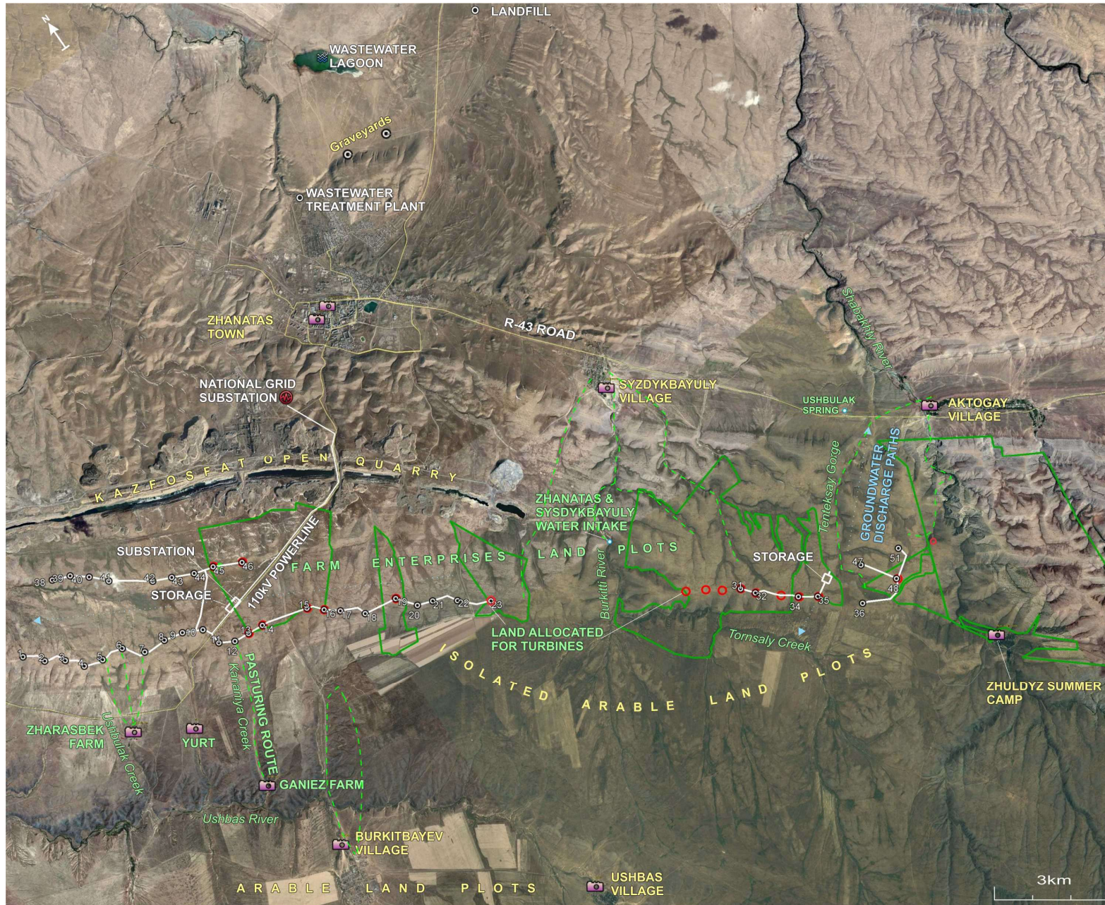
Figure 2 Overview of the wind-farm area. Project components are written in white, social constraints are shown in green. Green dash lines are pasturing routes. See Figure 6 for visual impact modeling from the identified sensitive viewpoints shown here as cameras.
