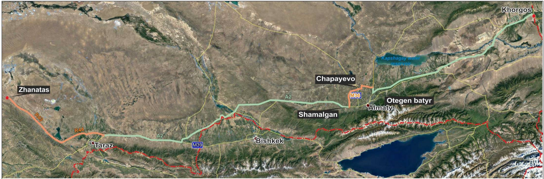
Figure 3 Windfarm parts road transportation route 1100km from Khorgos. Four lane roads shown in green, two lane roads – in pink where the route also has steep (12%) rises and descends. Turns that may require infrastructure alteration are framed black. The potentially constraining structures such as gates, overhead powerlines, above-road gas pipelines were located during a reconnaissance survey but bridges integrity and maximum allowed load is still to be assessed.
