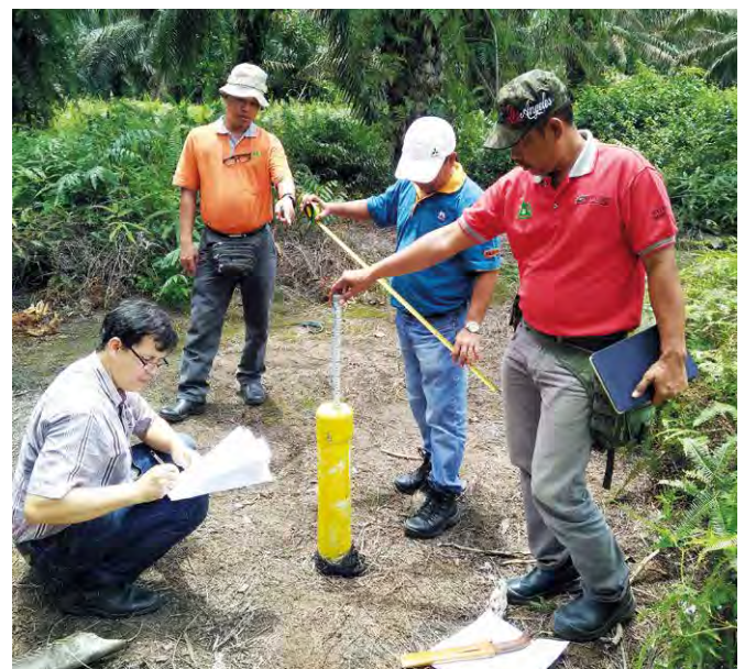
Ground water-table monitoring using a piezometer
