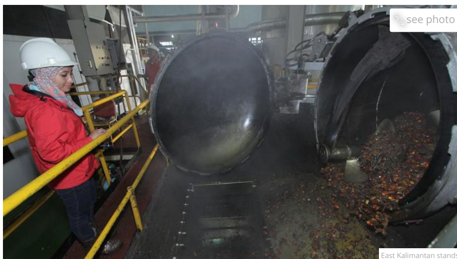
One of the production processes of Crude Palm Oil (CPO), with this machine the fruit and palm bunches are boiled, the aim is to kill the enzyme content in the oil bunches. This enzyme affects the acidity level of CPO.
