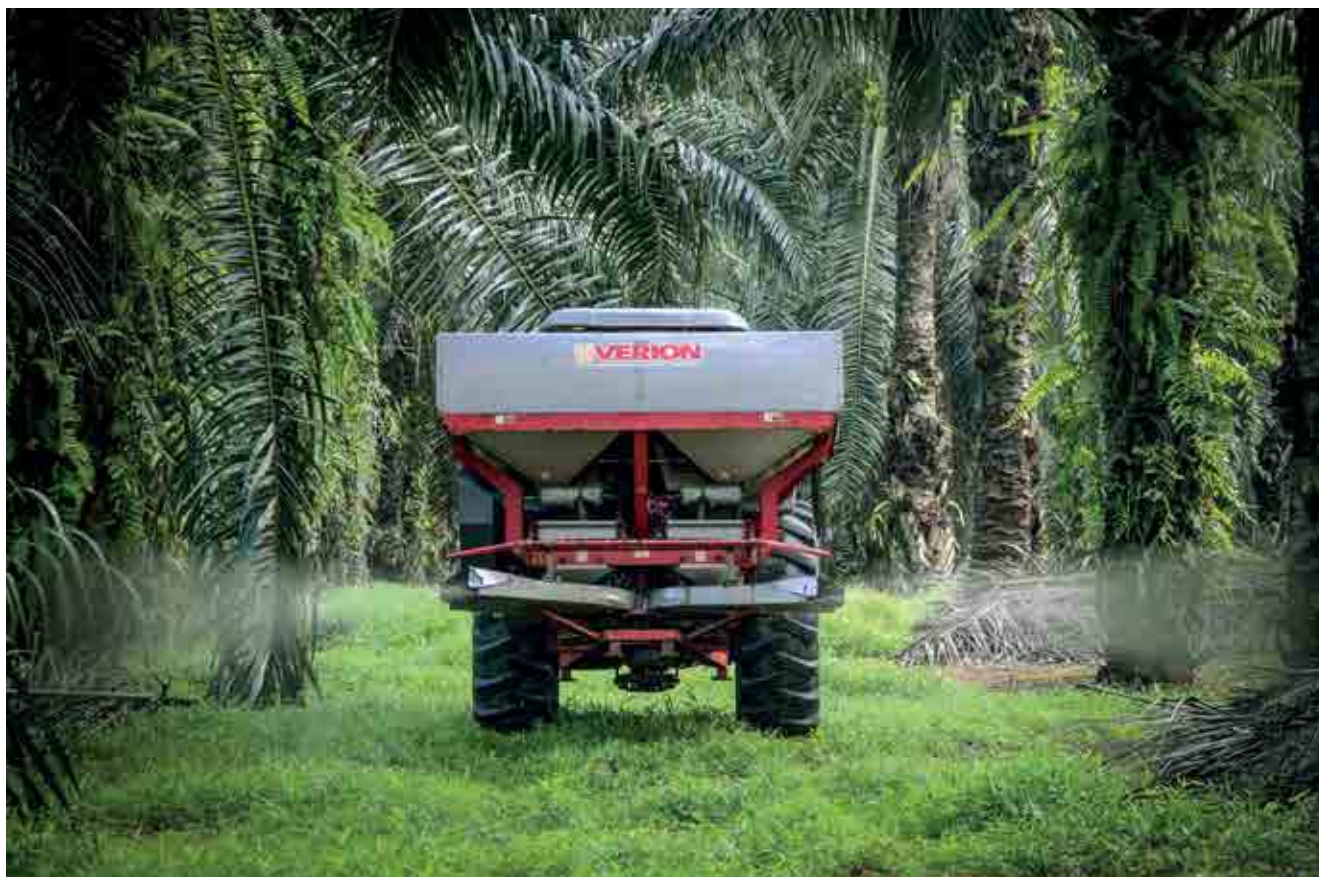
The Verion Smart Fertiliser Spreader is capable of applying 2 types of fertilisers in a single pass. Data collected autonomously by the machine can be used to produce an "As-Applied Fertiliser Map" to ensure that every palm obtains its fair share of recommended fertilisers
